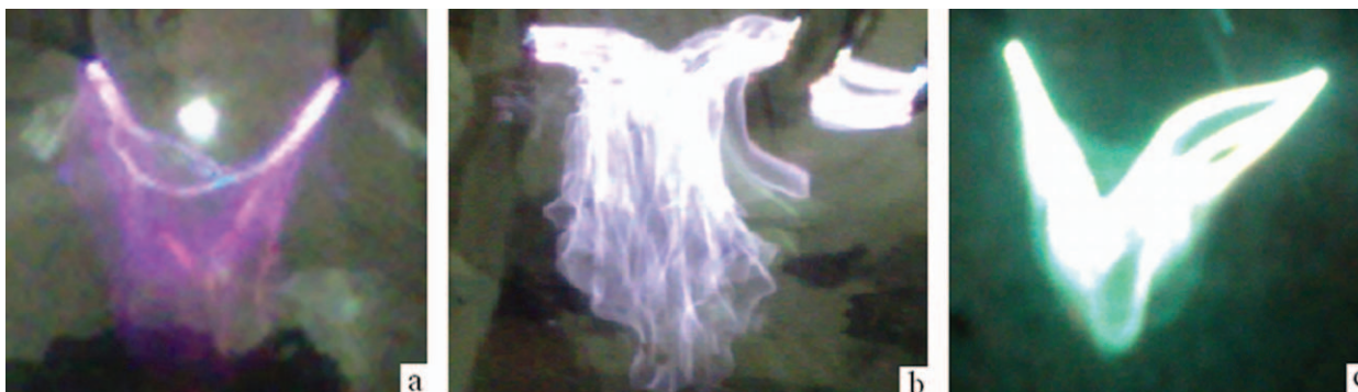
Figure 2. Photographs of MWCNTs treated by different plasma flame (a) air, (b) argon, and (c) styrene (argon is used as carrier gas). [Color figure can be viewed in the online issue, which is available at wileyonlinelibrary.com .]
